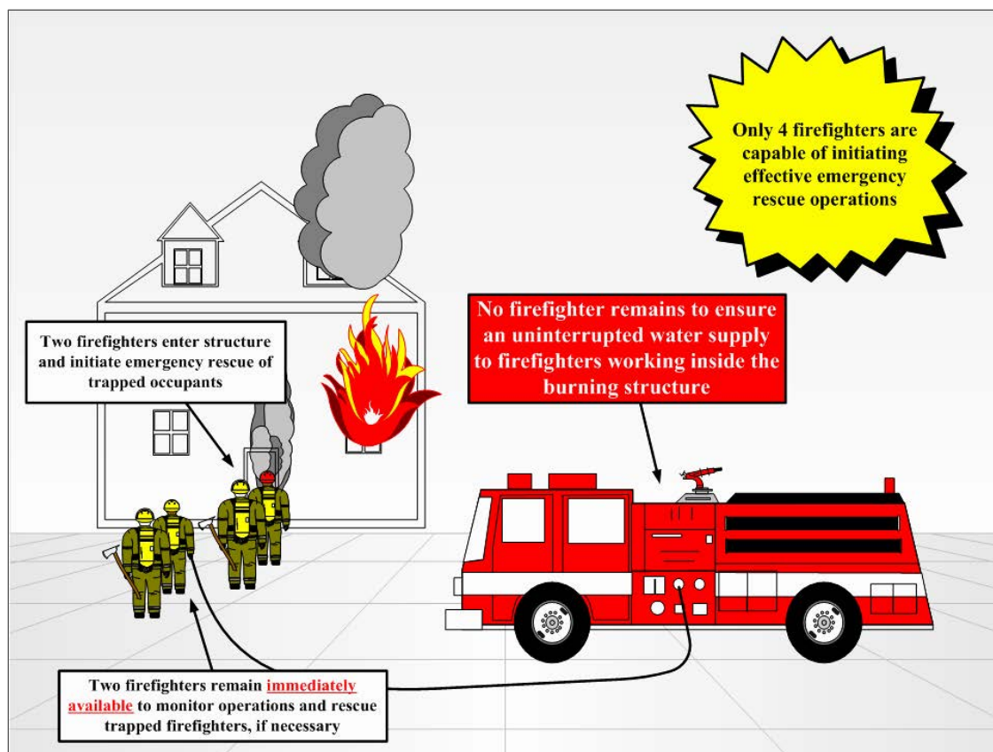
FIGURE 5-2: Two-In/Two-Out Interior Firefighting Model*
